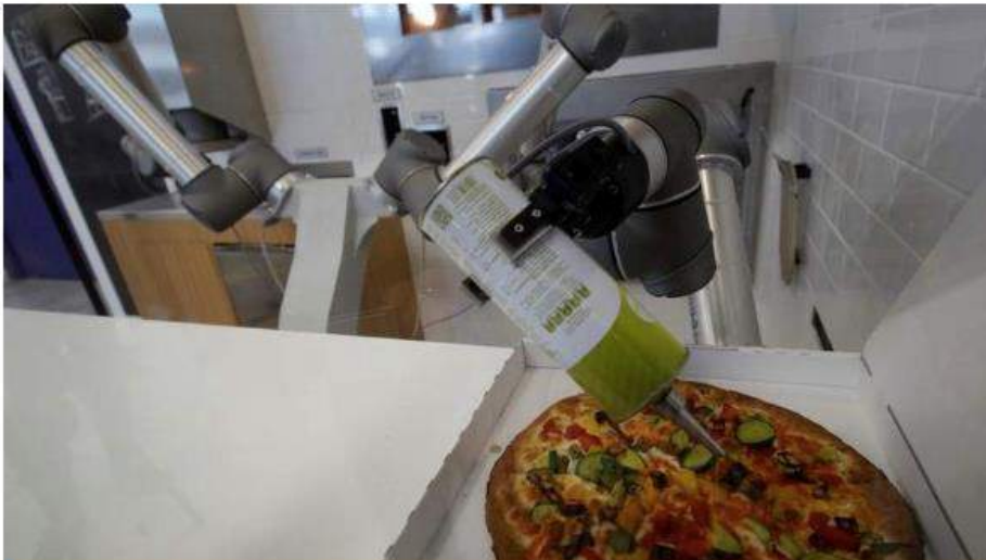
Ekim has three arms, can coordinate tasks and make several pizzas at once; one pizza takes four minutes and 30 seconds to
